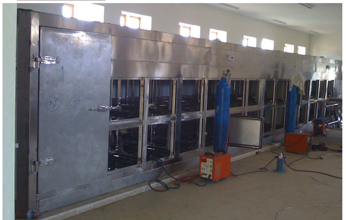
Firing Chamber set made of stainless steel 304
