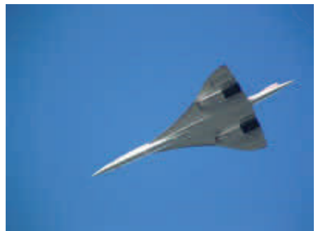
Concord jet's body, rudder and nose are made of Stainless steel
